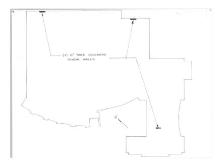
*Figure 10: Location of the three shear walls designed to resist the* lateral loads.
