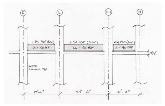
Figure 9: Sketch of analyzed frame with dimensions and loads.
