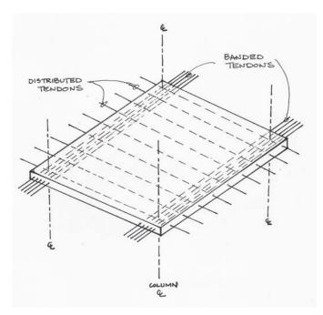
Figure 7: Typical post-tensioning tendon layout.
